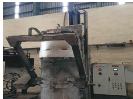
Electrical heater introduced in place of diesel burner
