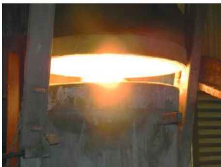
Electrical heater introduced in place of diesel burner
