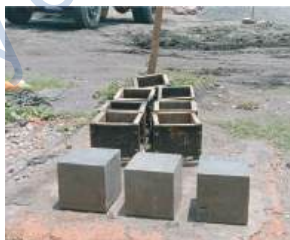
Concrete cubes casted for testing
